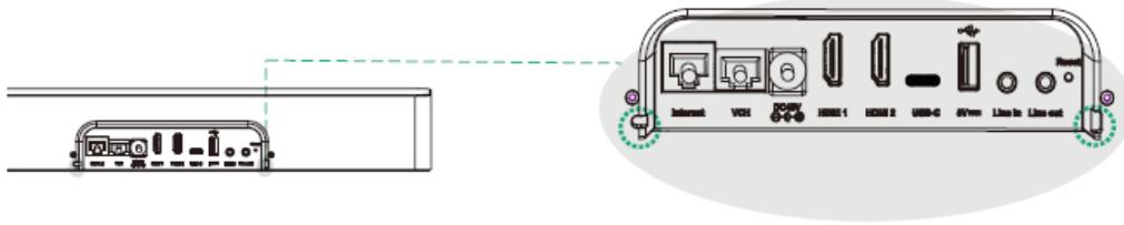
2 Fit part A of the cable cover into the slots.
